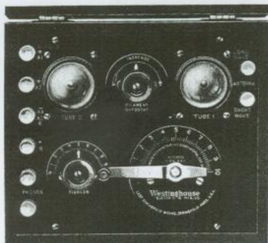
Fig. 5—Close-up of Panel
