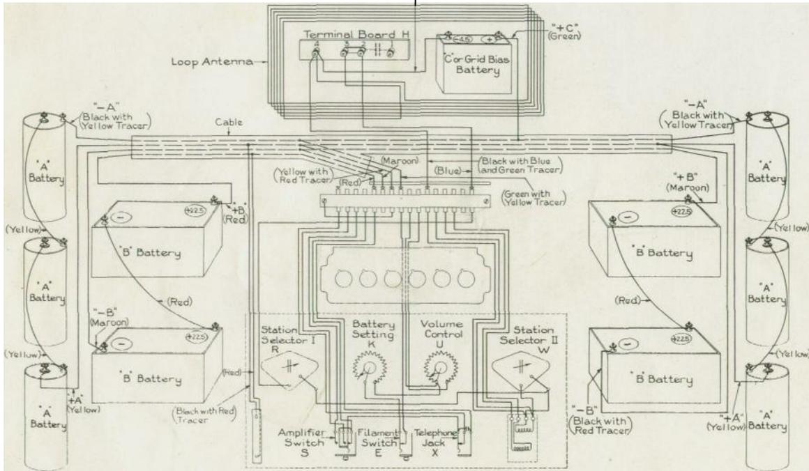
Fig. 6. Connection Diagram of Radiola Super-Heterodyne
