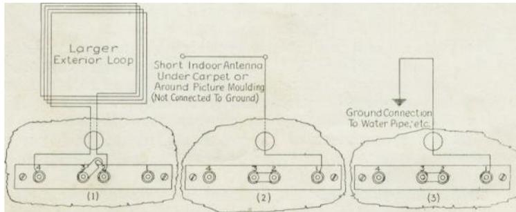
Fig. 6. Connection of Exterior Loop, Indoor Antenna, etc.
