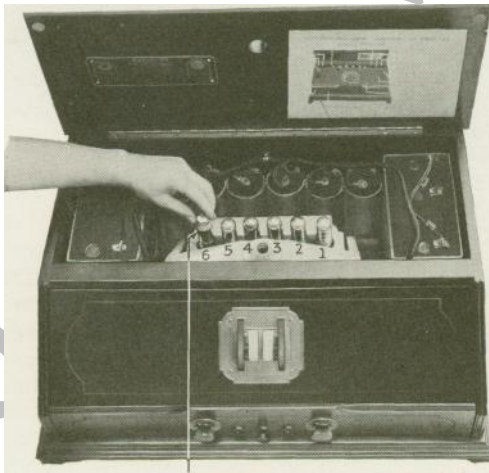
Insert Radiotron UX-120 in Socket 6 Only
