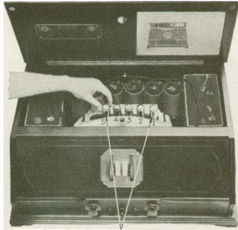
Insert Five Radiotrons UX-199 in Sockets 1 to 5
