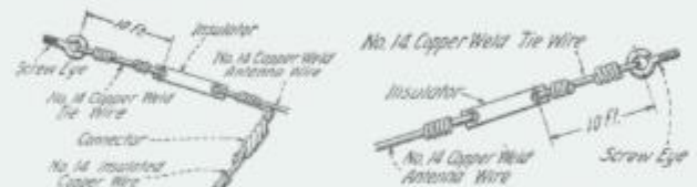
Fig. 2—To the left shows method of connecting the antenna to the lead-in wire. To the right shows the free end of the antenna and manner of fastening to support.
